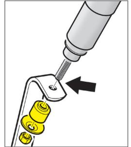
3. Attach the steering rack to the new front axle using the Original Hardware.
