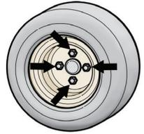
5. Remove the hub caps (if any). Loosen the lug nuts on both rear wheels but do not remove them.
