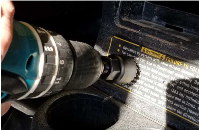
EC-022020 REV B – Use larger drill from 1" to 1-3/8" diameter
